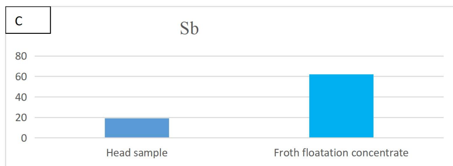
Figure 5. Histograms showing the values of head samples and concentrates (A-C); note the upgradation in values of Fe, Cu and Sb (wt.%).
